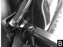
Step 5: Latch is left loose so you can adjust as needed. Latch door shut and tighten upper hinge bolts until snug. Check that door shuts and opens without interference. Adjust and tighten. Once adjusted, torque hinge bolts to factory specifications. (Figure C)
