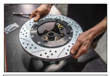
1. Start by inspecting the 4 mounting bosses on the hub and making sure they are clear of rust, debris, etc. Place the correct side rotor (Driver front shown) onto the hub and line up the 4 holes.
