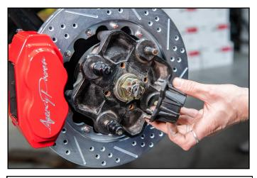
10. Finally re-install the factory dust cap by inserting the tabs into the hub face and snapping the 4 tabs into the holes.
