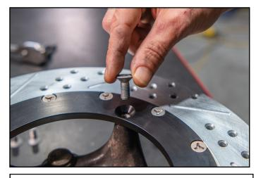
2. Use the supplied M8 x 20 FHCS bolts and apply a small amount of Blue Loctite on each bolt.
