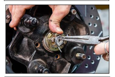
7. Install the cotter pin and bend one side on top of the axle end. Bend the other side down and away towards the hub face.
