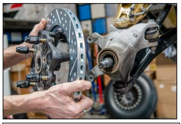
4. Next install the rotor/hub assembly onto the spindle by inserting the axle onto the splined portion of the hub. Now is a good time to inspect the outer seal, and replace if needed. Apply synthetic grease (XPS 293550010 or equivalent) around the drive shaft & splines. Be careful not to damage the outer bearing seal while installing the hub snout into the bearing. (Front Driver shown)
