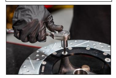
3. Using a 5mm allen head socket, tighten the bolts by hand. Tighten in a cross sequence to ensure the hat is flat to the hub. Once done torque these bolts to 25ft lbs.
