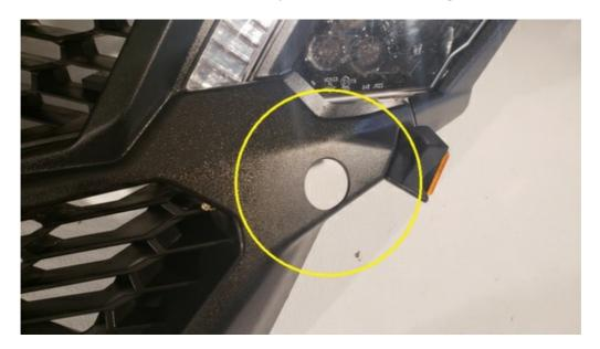
2. Install the front bumper over the (4) front control arm bolts and loosely install the original nuts, do not tighten. Make sure the lower radiator mounting tabs lay behind the corresponding mounting tabs on the front bumper.
