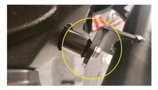
4. Secure the rear mounting tabs of the left and right support bars to the unused holes in the vehicle's frame just above the rear upper control arms using (1) M8x20 Hex Bolt, (1) 5/16" Fender Washer, (1) ¼" Washer, and (1) M8 Nyloc Nut for each side. The 5/16" Fender Washer will go against the head of the bolt then pass the bolt through the rear of the frame and support arm followed by the ¼" Washer and Nyloc Nut.
