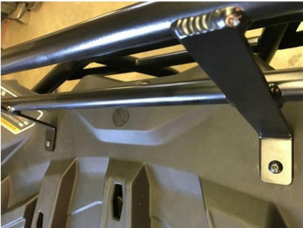
4. Line up the previously installed clamps with the cargo rack and install the supplied allen head bolts.
