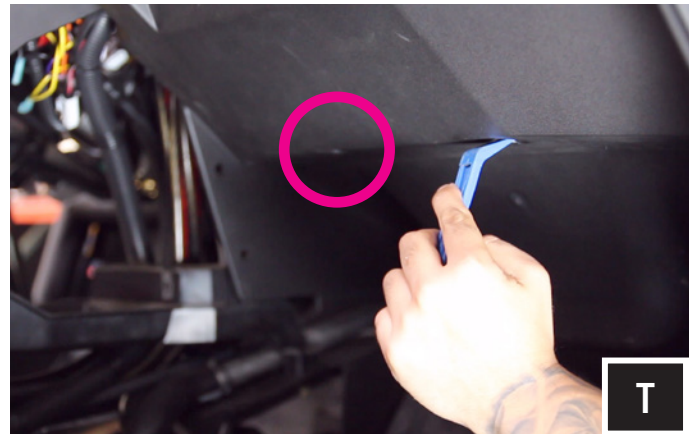
T. Remove push clips from underneath glove box.
