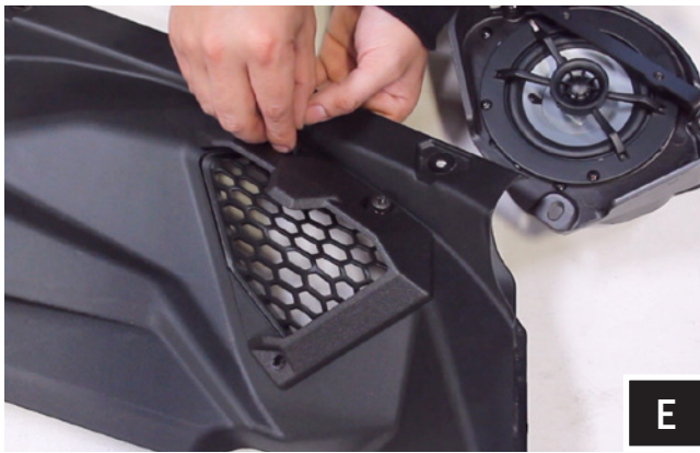
E. Place the acoustic lens on top of the factory grille, line up the holes and insert the (2) top M6x16mm (shorter) screws and washers.
