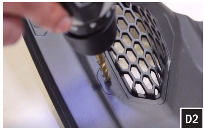
D. Drill a hole using a 1/4" drill bit at the factory dimple marks (as shown above) on the outside dash panel around the speaker grille.
