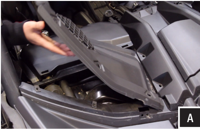
A. Remove the top dash panels on the driver (7 screws with 2 clips) and passenger side (5 screws with 2 clips). Be sure to lower the steering column and remove the two bolts from the instrument cluster and pull the cluster loose in order to get this panel out.
