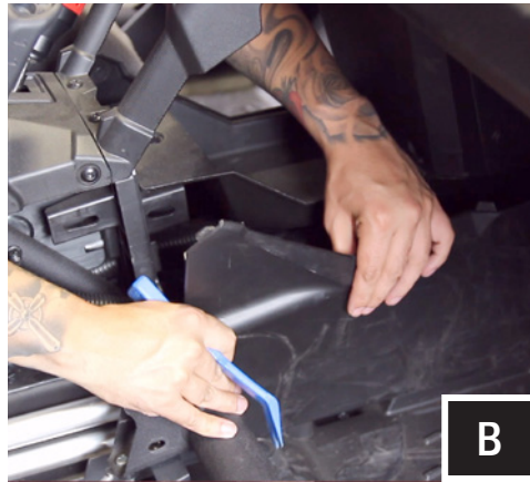
B. Carefully unsnap console panels by hand or with a panel removal tool.
