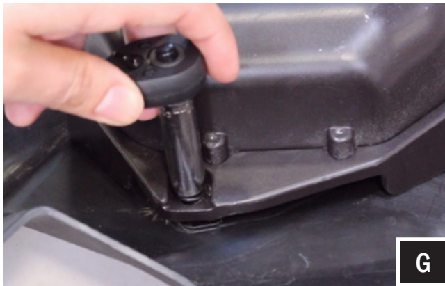
G. Insert the M6x25mm screw by pushing it through the acoustic lens, dash panel and speaker pod. Secure screw using washer and 10mm nut. Now fasten the previous (2) M6x16mm screws.
