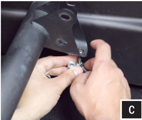
C. Remove the factory 10mm nut and bolt from the brake line. Place the washer on top of the factory bracket and push the long M6x25mm screw through the top. Then attach the brake line, spacer, washer and nut. (Disregard this step for the 4-seat Maverick X3 Max)
