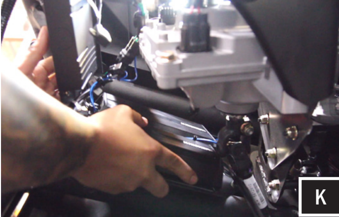
K. From underneath driver side place amp plate between the two cross bars behind the steering wheel.
