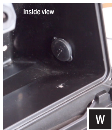
W. Unscrew and remove the plastic nut from the port. Make sure to open the fuse holder and remove the fuse so the nut will fit through it. Feed in the wires through the hole. Keep the fuse holder open and empty until it has passed through the hole.
