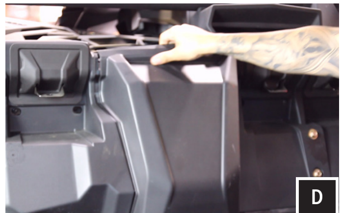
D. Carefully unsnap rear cover to expose the engine compartment
