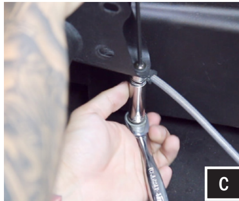
C. Remove the factory 10mm nut and bolt from the brake line. Place the washer on top of the factory bracket and push the long M6x25mm screw through the top. Then attach the brake line, spacer, washer and nut. (Disregard this step for the 4-seat Maverick X3 Max)
