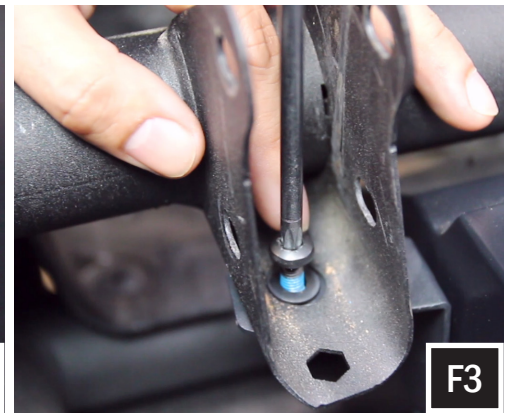
F. Place B-Bracket to the left side of the enclosure and slide the tab underneath the enclosure. (F1) Line up the 2 screw holes and proceed to hand thread the M6 screws and washers. Use a T30 Torx bit to tighten screws. Repeat for the right side. (F2) Line up the top of bracket A and B with the holes on the factory seat bracket. Screw in the M6 screw with the large washer (F3).
