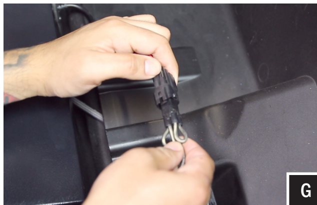
G. Route the speaker wire away from any moving parts and any sharp metal, then connect to the amplifier. Connecting the X3-US10 using the pre-installed, four-pin connector will require an optional SSV Works plug-&-play harness B-H1152 - sold separately).
