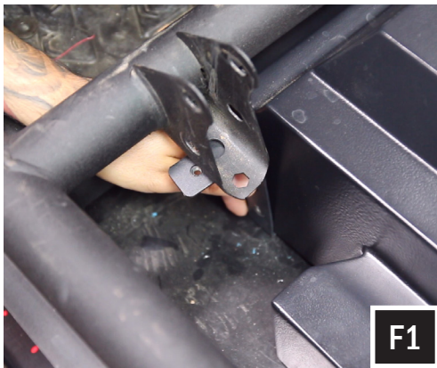
F. Place B-Bracket to the left side of the enclosure and slide the tab underneath the enclosure. (F1) Line up the 2 screw holes and proceed to hand thread the M6 screws and washers. Use a T30 Torx bit to tighten screws. Repeat for the right side. (F2) Line up the top of bracket A and B with the holes on the factory seat bracket. Screw in the M6 screw with the large washer (F3).
