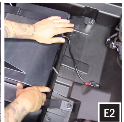
E. Run the brake line along the dedicated channel on the sub enclosure while feeding the enclosure down under the seat bar (F1). Make any adjustments to the brake line so the enclosure lays on top of it. Line up the rear enclosure brackets to the rear seat bolts and press down until the brackets rest on top of the spacers.
